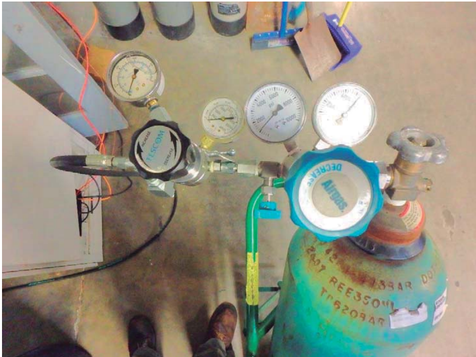
Figure 12: Proof and burst pressures test setup – air source
