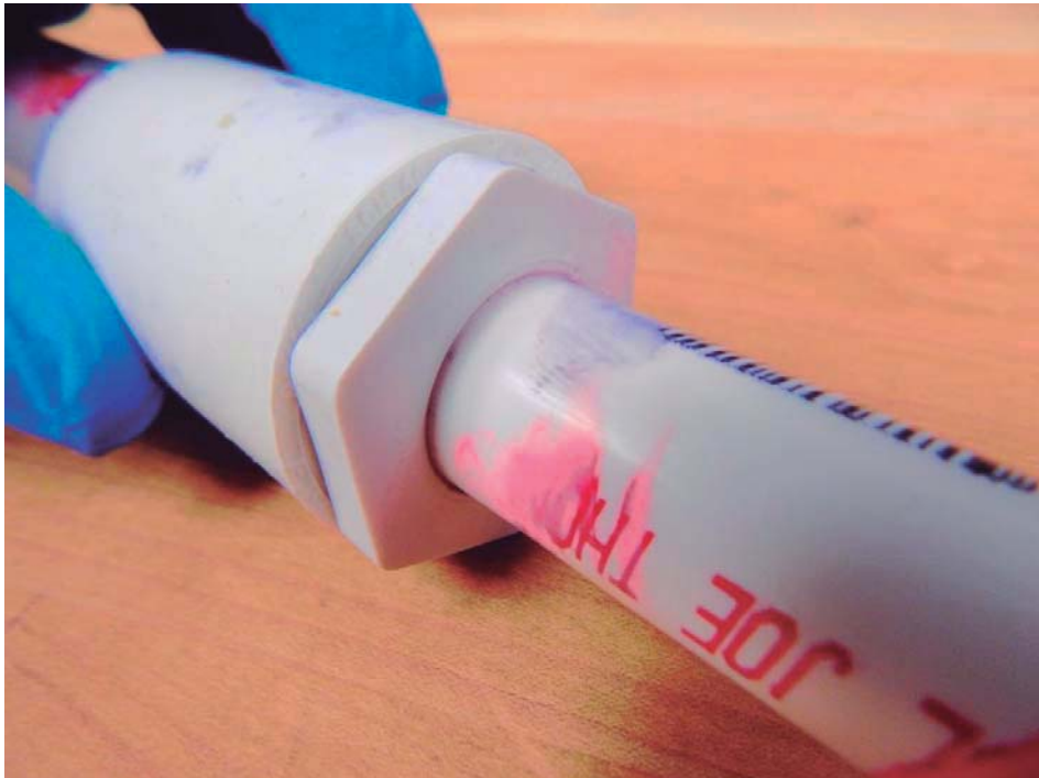
Figure 20: Test hardware after testing – leak area
