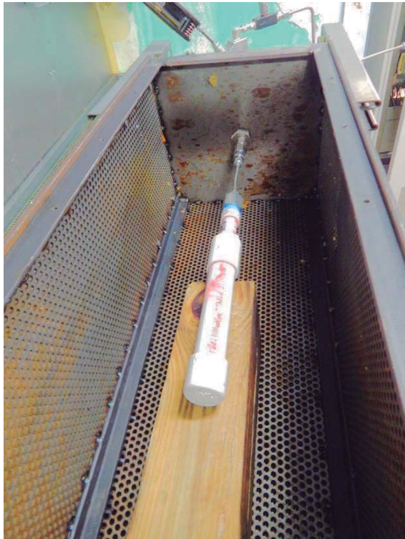
Figure 7: Proof and burst pressures test setup – test hardware installed in test setup
