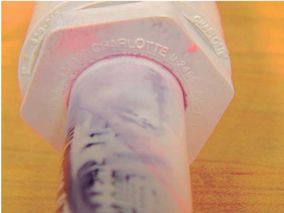
Figure 22: Test hardware after testing – leak area
