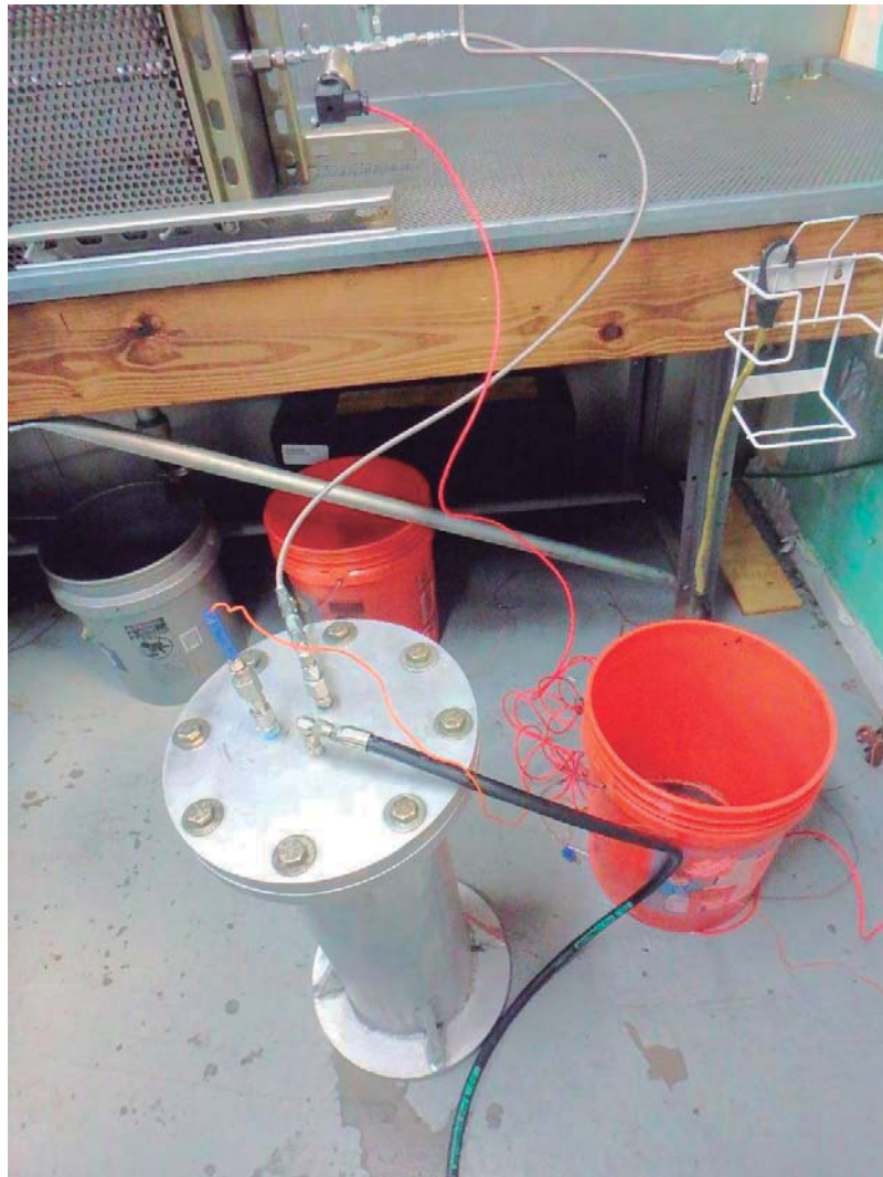
Figure 10: Proof and burst pressures test setup – air and water vessel
