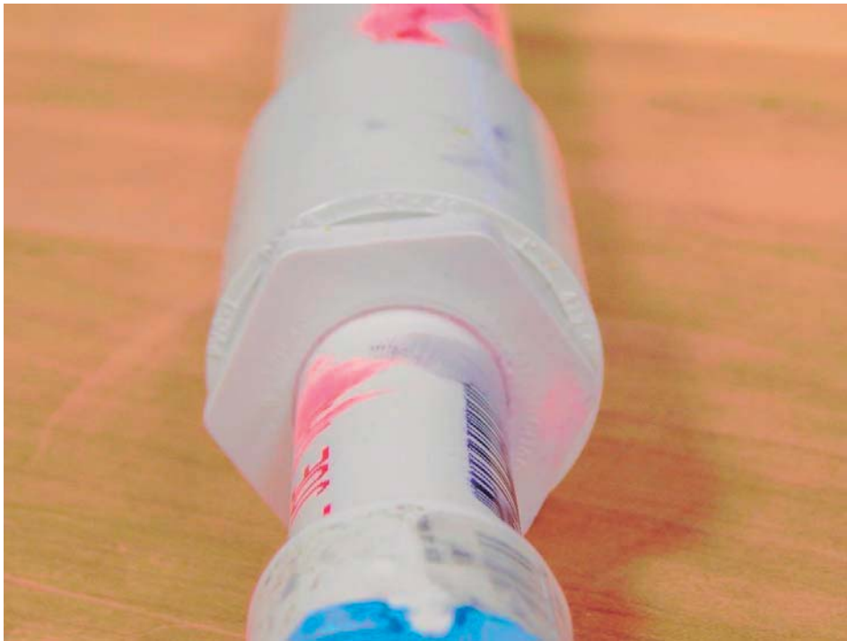
Figure 23: Test hardware after testing – leak area
