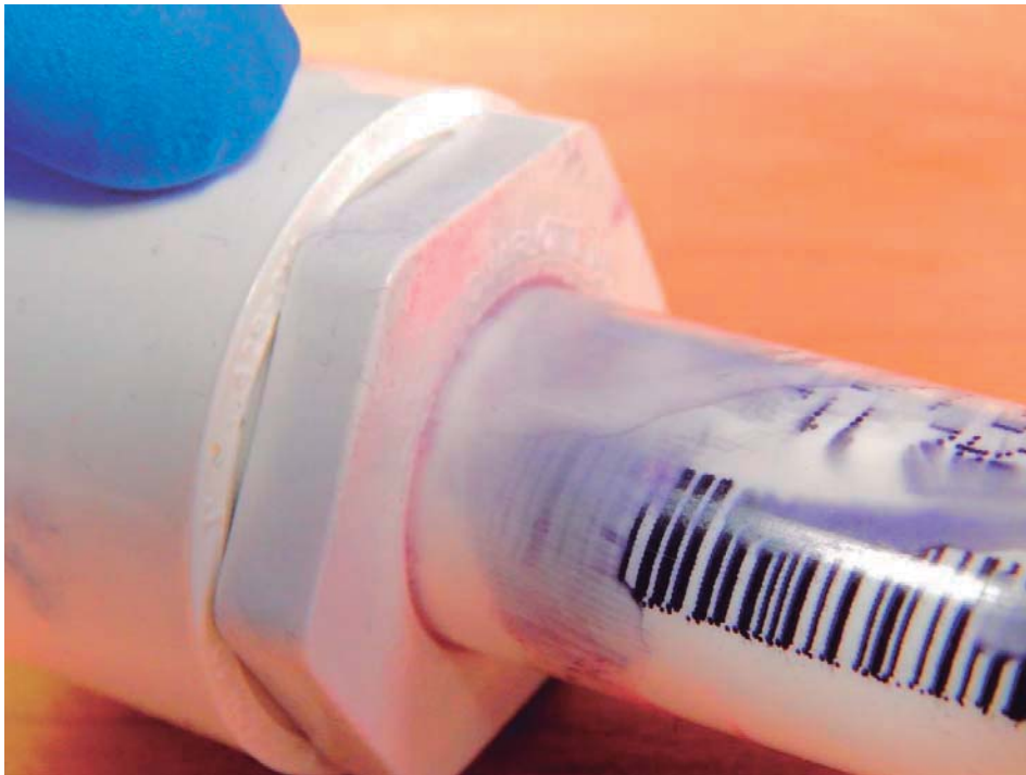
Figure 21: Test hardware after testing – leak area
